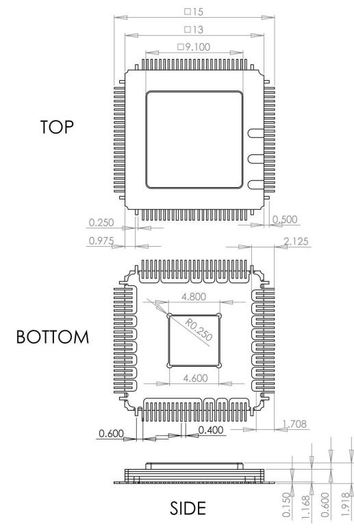
Fig. 6. CQFP 100-Pin Package Drawing (All Dimensions in mm)
