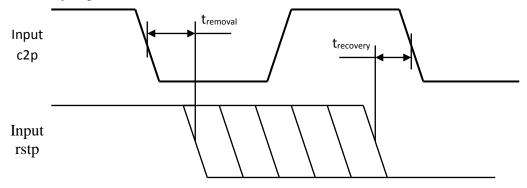
Fig. 3. Reset Timing Diagram
