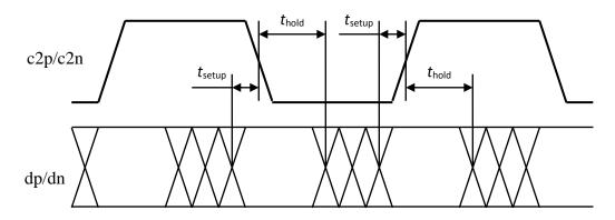
Fig. 4. Input Timing Diagram
