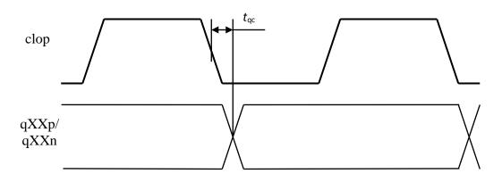
Fig. 5. Output Timing Diagram
