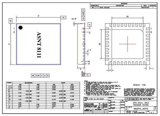
Fig. 3. QFN 40-Pin Package Drawing (All Dimensions in mm)
