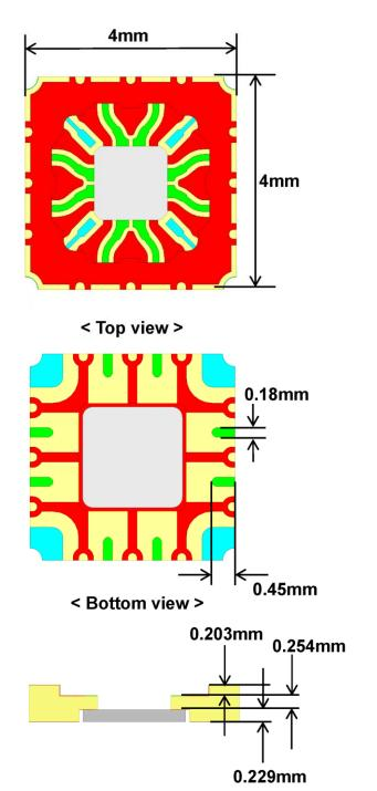
Fig. 3. CQFN 24-Pin Package Drawing (All Dimensions in mm)
