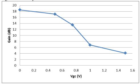
Fig. 2. Single-ended Gain vs. Vgc
